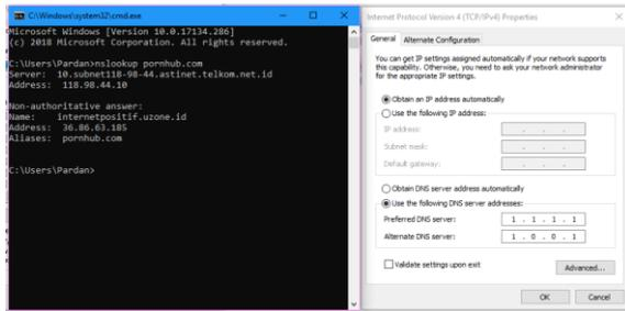
**Figure 14** Changing DNS Settings With Transparent DNS
