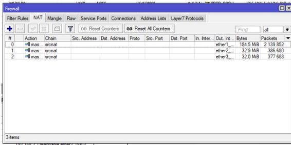
Figure 7 NAT Firewall IP Configuration
