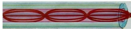
Gambar Error! No text of specified style in document.-5. Multi Mode Fiber
