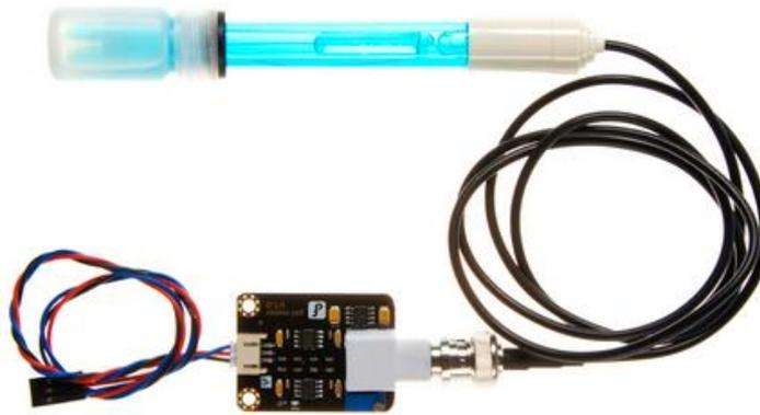
**Gambar 2.5 Sensor pH Meter**
