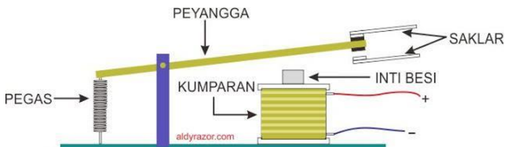
Gambar 2. 6 Prinsip Kerja Relay
