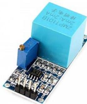
**Gambar 2.15** Sensor Tegangan ZMPT101B
