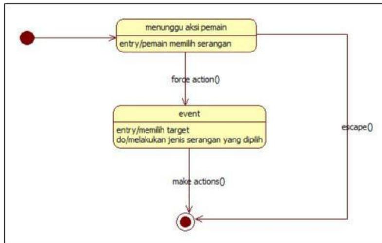
**Gambar 2.5 State Machine Diagram**
