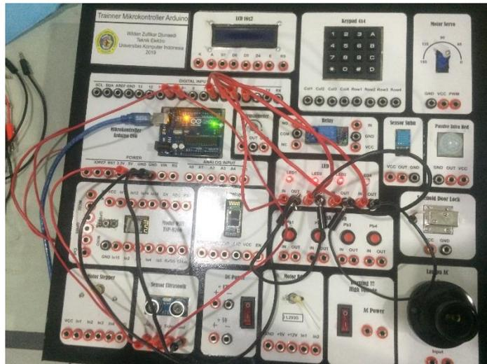
**Gambar 4. 25** Uji coba Rangkaian Sensor Jarak
