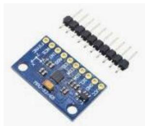
*Gambar II-12 Accelero-Gyro Module MPU 9250*
