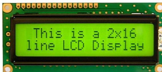
Gambar 2.7 Liquid Crystal Display
