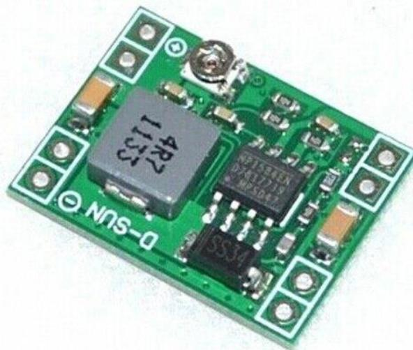
**Gambar 2.13 – Step Down Module**
