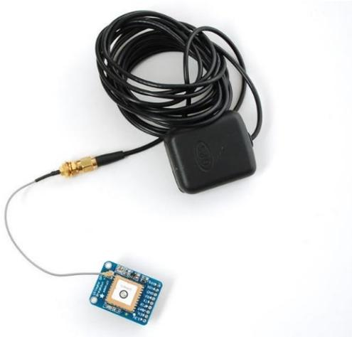
**Figure 6. Module GPS Antenna**
