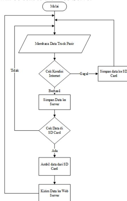
Figure 2. IOT Tool Workflow Analysis
