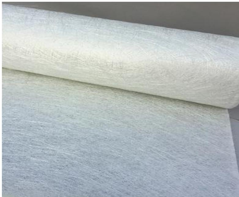
Gambar 2.16 serat gelas (fibre glass)
