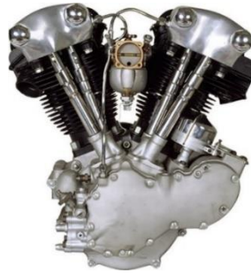
Gambar II. 6 Mesin Harley Davidson Jenis Knucklehead Tahun 1936 – 1947 Sumber : https://www.gridoto.com/amp/read/221035578/evolusi-mesin-harley-davidson-dari-masa-ke-masa-dari-yang-imut-hingga-gempal (05/04/2024)
