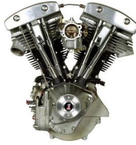
Gambar II. 8 Mesin Harley Davidson Jenis Shovelhead Tahun 1966 – 1984 Sumber : https://www.gridoto.com/amp/read/221035578/evolusi-mesin-harley-davidson-dari-masa-ke-masa-dari-yang-imut-hingga-gempal (05/04/2024)
