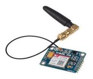
Figure 4 Module SIM800L
