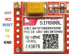
**Gambar 2. 11** Modul GSM SIM 800-L
