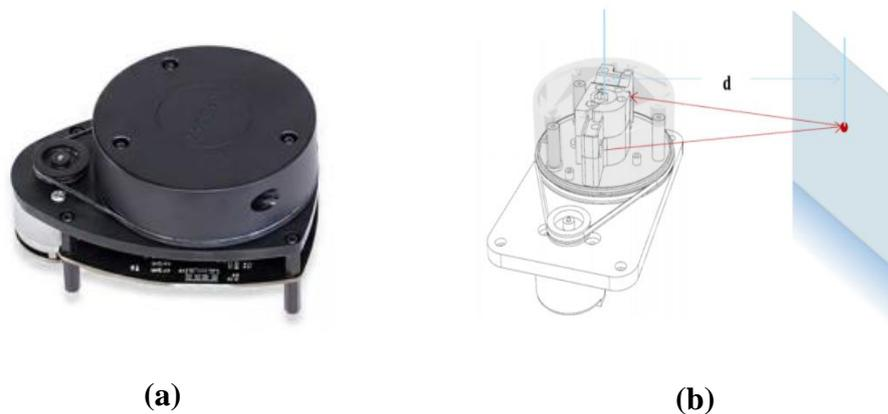
**Gambar 2.7.** (a) Sensor RPLidar A1M8, (b) Prinsip Pengukuran [14]
