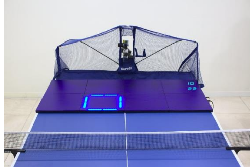
Gambar 2.1: Robot Pelontar Bola Pingpong Interaktif FastPong [1]
