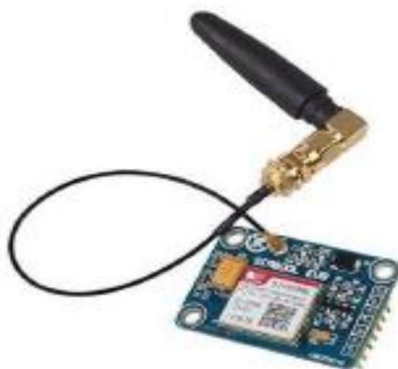
**Gambar 2.10 Modul GSM SIM800L V2**
