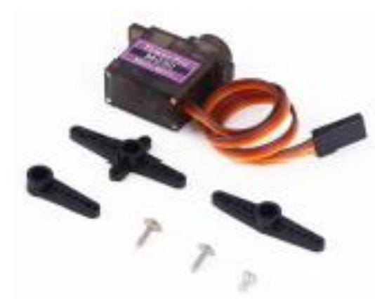
**Gambar 2.9 Motor Servo MG90**
