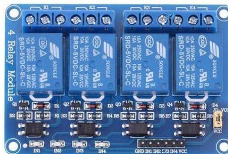
Gambar 2. 7 Relay 4 Channel
