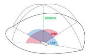
Figure 1. Area Coverage Leap Motion Controller
