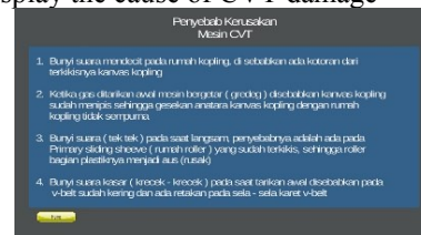
Figure 12 Display the causes of CVT damage
