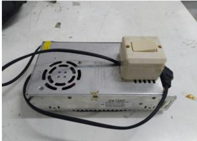
Gambar 2. 9 Power Supply 12V 30A
