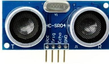
Gambar 2.5 Sensor Ultrasonik
