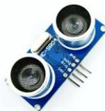
**Gambar 2.22 Modul Sensor *Ultrasonik* HC-SR04**
