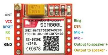
**Gambar 2.25 Modul GSM SIM800L**
