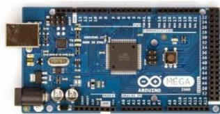
**Gambar 2.12 *Arduino Mega***
