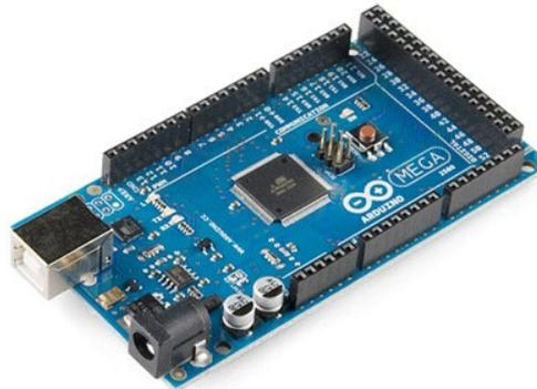
Gambar 2. 5 Arduino Mega 2560
