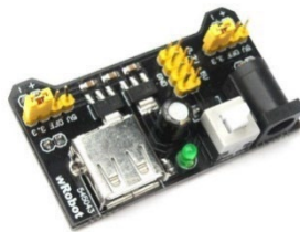
Gambar 2.8 PSU Dual Voltase
