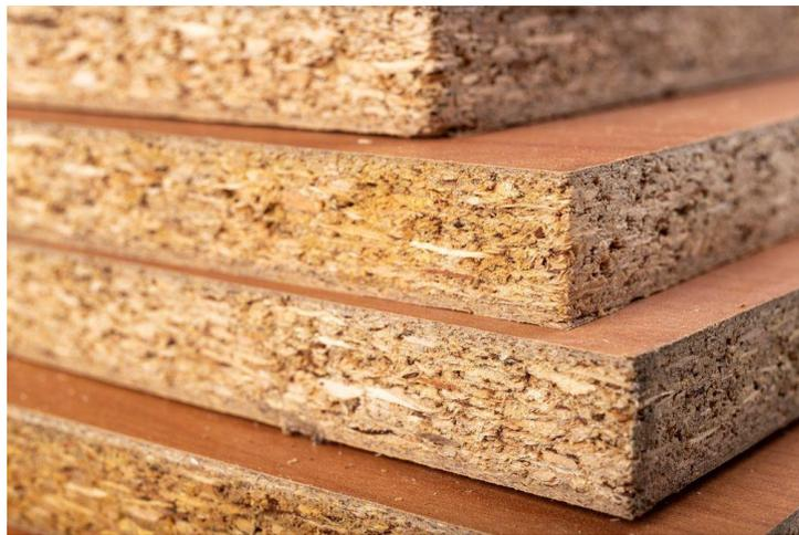
*Gambar 2.13 Particle Board*
