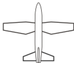
Gambar 2. 9 Compound Tapered Wing
