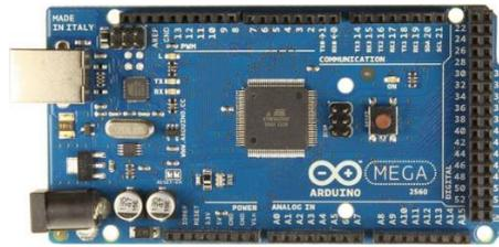
Gambar 2.3 Arduino Mega 2560
