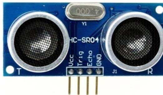
Gambar 2.7 Sensor Ultrasonik
