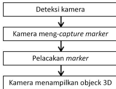
Figure 2. Marker Based Tracking Flow Method
