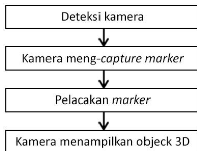
Gambar 2. Alur Metode Marker Based Tracking
