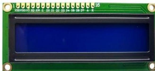
**Gambar 2. 9** *Liquid Crystal Display*
