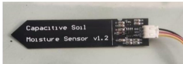
Gambar 2.11 Sensor Capacitive Soil Moisture .
