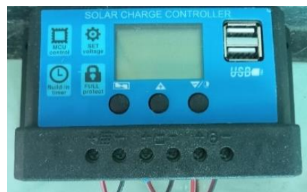
Gambar 2.17 Solar Cell Charger.
