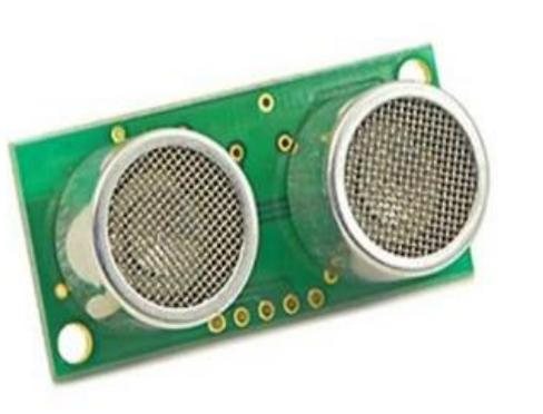
**Gambar 2.15 Model sensor Devantech SRF04**
