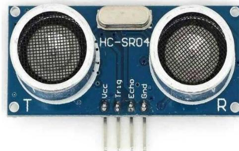
**Gambar 2.14 Model sensor parallax Type HCSR04**
