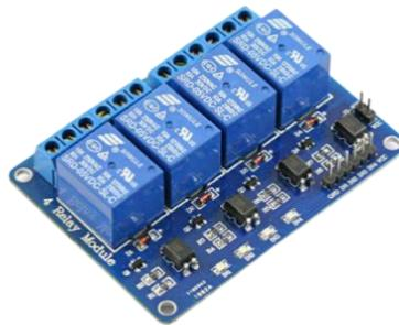
**Gambar 2.7.1** Modul Relay 4 Channel.
