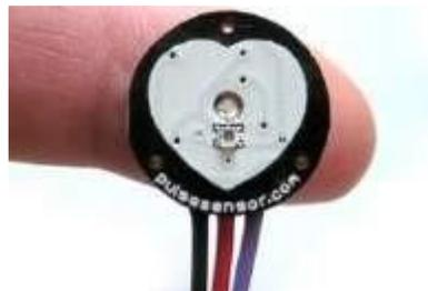
*Gambar II- 6: Pulse Sensor*
