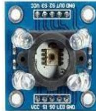
Gambar 2.2 Sensor Warna TCS3200
