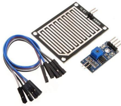
Gambar 2.35 Sensor Raindrop FR-04
