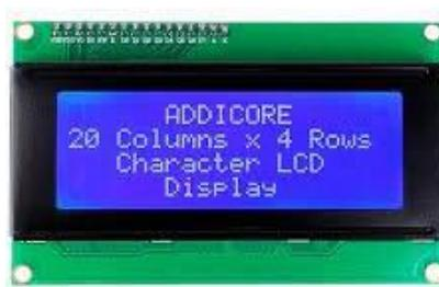
**Gambar 2.4 LCD (*Liquid Crystal Display*)**
