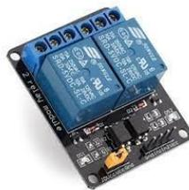
**Gambar 2.10 Modul Relay 2 Channel**
