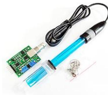
Gambar 2.20. Sensor pH PH4502C
