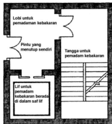
Gambar 2. 4 Denah Lift Kebakaran (Sumber: PERMEN No.26)
