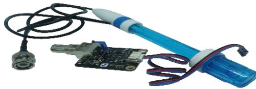
*Gambar 2.1 Sensor pH Air*
