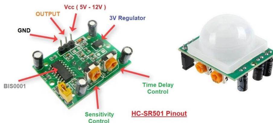
Gambar 2.6. Modul Sensor PIR (*Passive InfraRed*) HC-SR501
