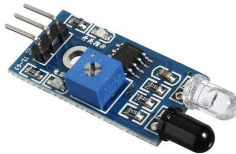
**Gambar 2.6** Infrared Obstacle
