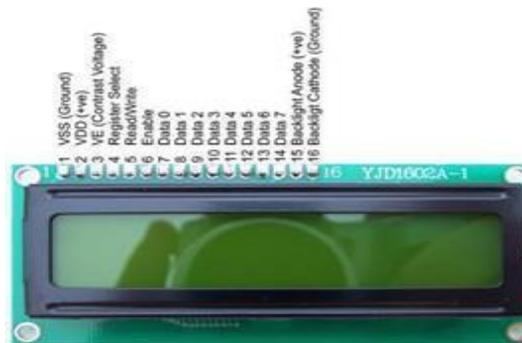
**Gambar 2.5** LCD 16x2
