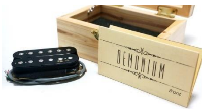
Black Open Coil Humbucker (50mm) Alnico V ; 12,60 kGhm ; 5,70 H 4 Wires Front / Neck Position
