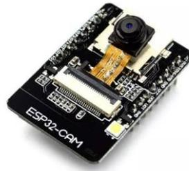
**Gambar 0.1 ESP32 CAM**
