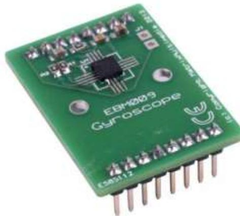
**Gambar 2. 7 Sensor Gyroscope**
