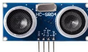
**Gambar 2. 15** Sensor Jarak HC-SR04
