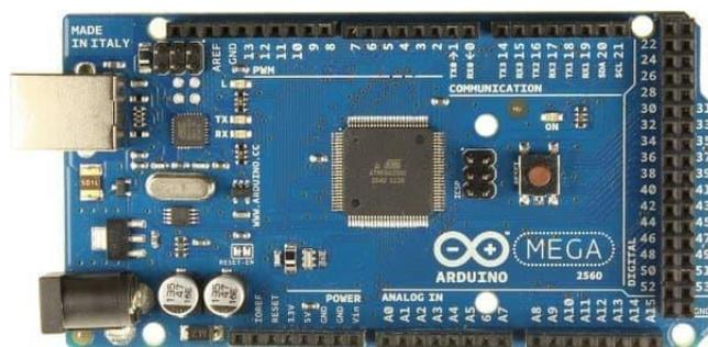
Gambar 2. 1. Arduino Mega 2560
