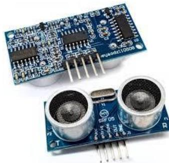
Gambar 2. 6. Sensor Ultrasonik HC-SR04
