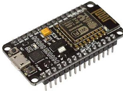
*Gambar 2.1 NodeMCU ESP8266 V1.0*
