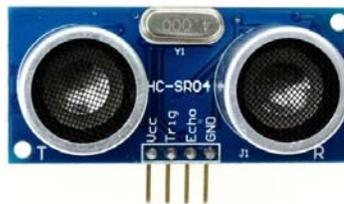
Gambar 2.4 Sensor Ultrasonik HS-SR04
